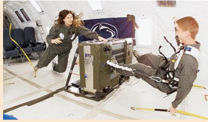
devised an active version of the device that can exert a constant force on a person who is exercising—just like on earth. The previous static version didn't create a constant force. "By doing deep knee bends with the device on board the plane in microgravity, we can test the system to its fullest," she says. "It was a proof of concept."
