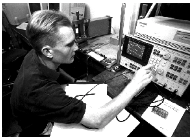
Christopher Davis measures the frequency response of a tunable vibration absorber.
