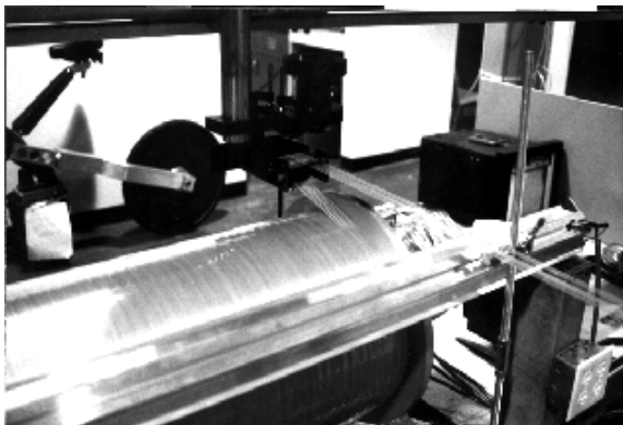
Bakis is currently perfecting a 300 pound flywheel, shown here during the filament winding, for use by a large midwest power company. The power company hopes to use the new flywheel to store energy at night when the demand for power is low. Power companies might also use such large flywheels on a neighborhood basis in substations to absorb and provide sudden power surges as demand changes from location to location.
