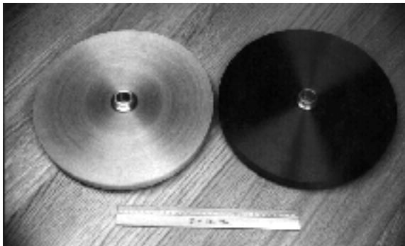
Two elastomeric flywheels wound directly onto hubs, fabricated for research purposes. The light one is a rotor made with a glass fiber filament, and the dark one is composed of carbon fiber filament.
