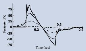
Waveforms calculated underwater from a surface-measured F-15 double-peaked wave at varying ocean depths. The solid line = 0 meters; short dashes = 4m; long dashes = 16m; and dash/dot line = 64m. The horizontal axis is time in seconds, the vertical axis is pressure in pascals.
