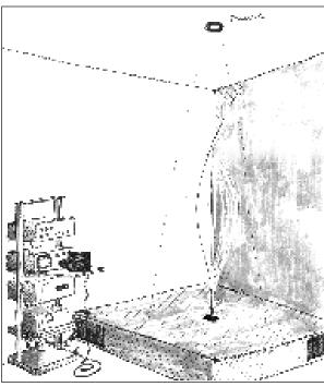
Cusumano's illustration for a publicly displayed kinetic sculpture, consisting of a single fiberglass rod about 10' high, and driven by an actuator hidden in the base. Wave forms are projected in real time onto the base from a projector in the ceiling, and sounds would come from speakers in the base corners (right side of illustration was cropped). Sensors, amplifiers, and video camera are on the rack to the left.
