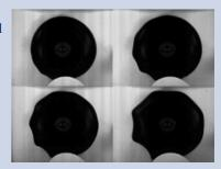
This sequence of photos shows the development of a standing wave in a tire as it passes a critical speed. The researchers in the nonlinear dynamics lab learned the cause of the standing wave and how to suppress it, making higher speeds possible.
