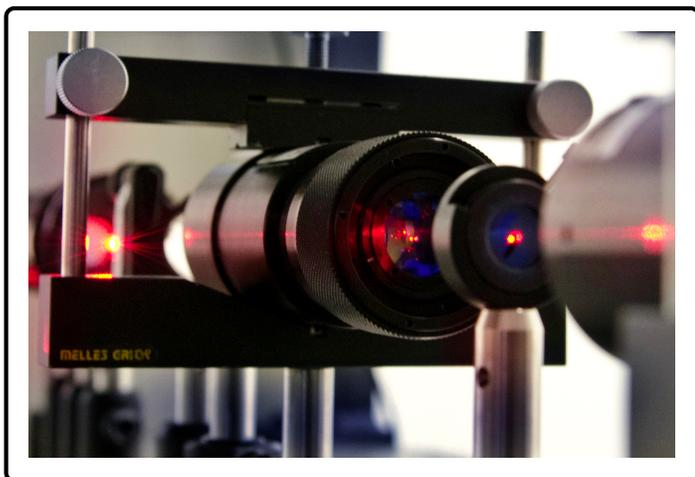
A demonstration set-up in Mohsen Kavehrad's lab creates partially coherent visible (red) light. This type of light performs better through the atmosphere than pure coherent light, an important consideration for outdoor optical wireless applications.
