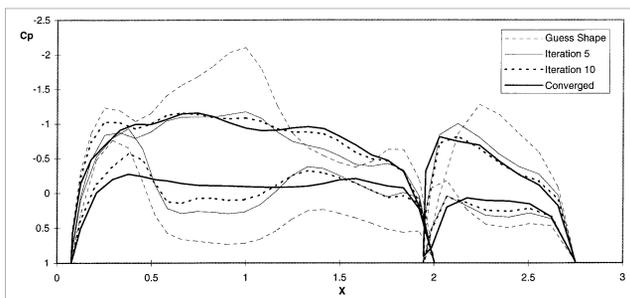
**The design software allows a guessed shape to be modified into a configuration that achieves a desired pressure distribution on its surface. The top screen shows evolution of geometry during the process. The bottom screen shows plots of the surface pressure distributions for the shapes above.**
