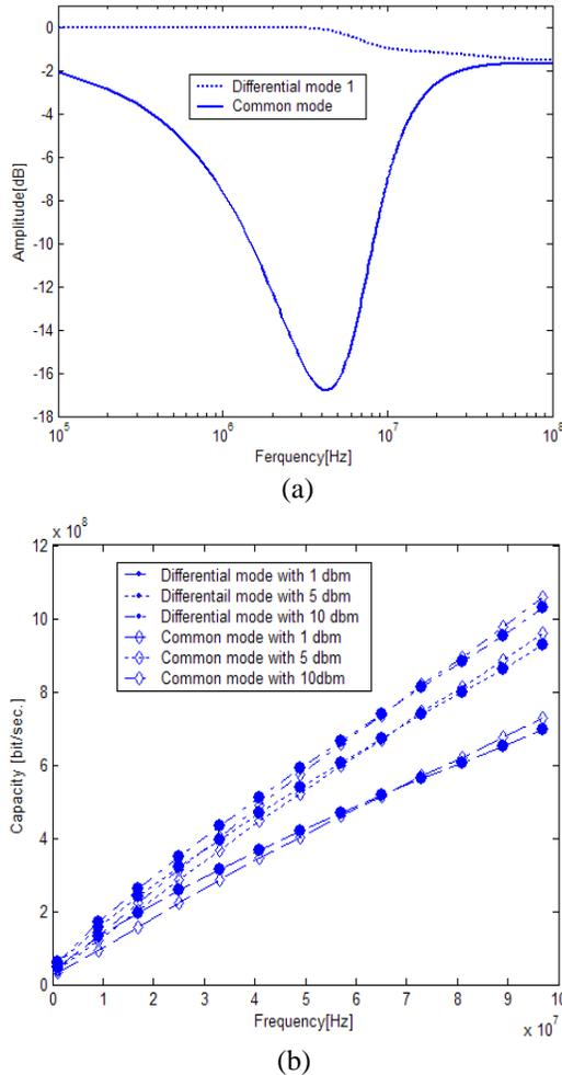
Fig.-3 (a) Frequency response of matched MTL transmission over 1 Km for differential and common modes coupling (b) Corresponding capacity values for different coupling methods and transmit power levels as a function of frequency band
