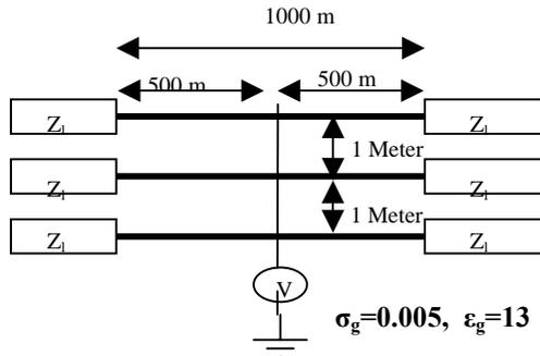
Fig.-5 Power-line configuration for radiation pattern simulations
