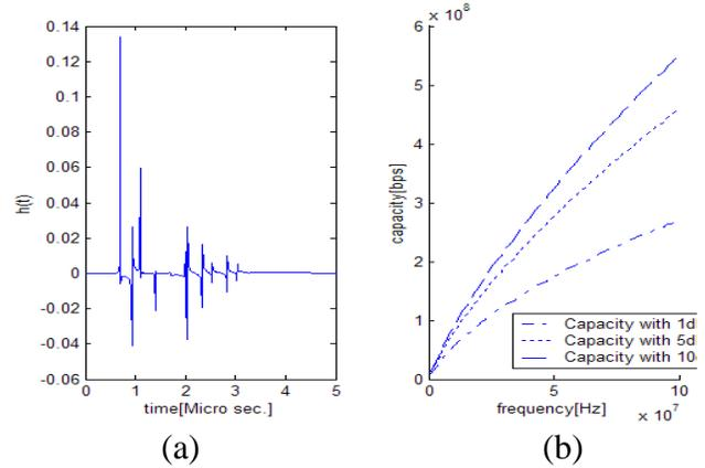
Fig.-4 (a) Channel impulse response of a complex network (b) Associated capacity values
