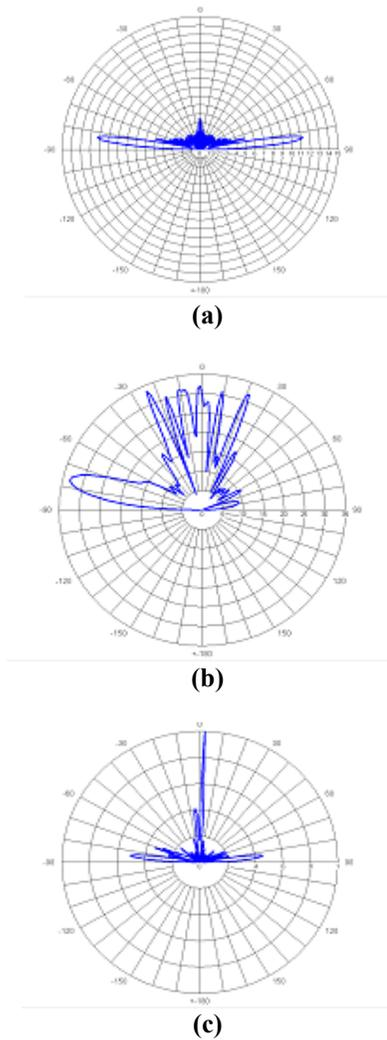
Fig.-6 Far field radiation from power-line configuration in Fig.-5, for (a) central common mode, (b) side common mode and (c) differential mode injections.
