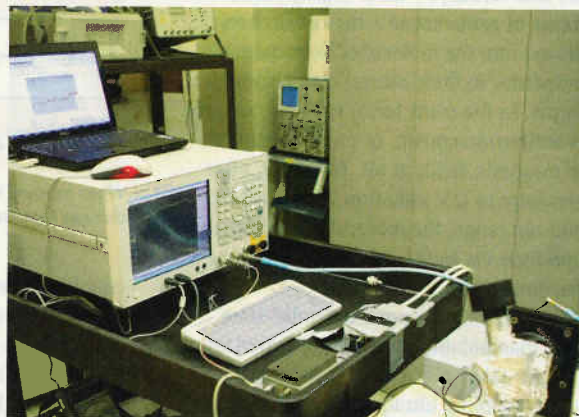
Pennsylvania State University researchers have developed a diffused light setup for optical wireless transmission with speeds exceeding 1 Gb/s.
