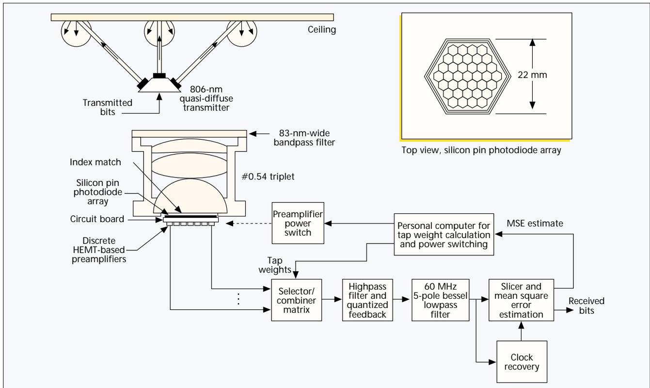
■ Figure 6. 100 Mb/s nondirected non-LOS infrared wireless link.
