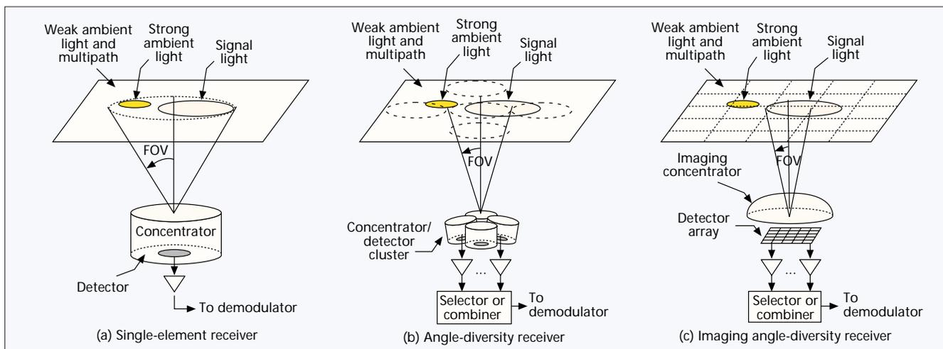
■ **Figure 1.** Types of free-space optical receivers. a) Single-element receiver, which may utilize non-imaging or imaging optics; b) angle-diversity receiver, which utilizes a collection of narrow-FOV elements, each equipped with a separate light concentrator, which are oriented in different directions; c) imaging angle-diversity receiver, which utilizes a single imaging lens and a photodetector segmented into multiple pixels.
