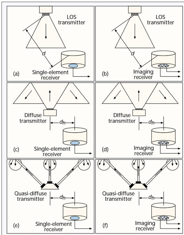
■ **Figure 2.** Types of free-space optical links, designated by transmitter/receiver types: a) LOS/single-element; b) LOS/imaging; c) diffuse/single-element; d) diffuse/imaging; e) quasi-diffuse/single-element; f) quasi-diffuse/imaging.
